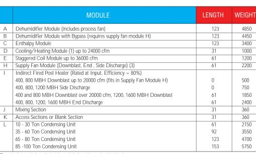
To calculate unit length total module lengths and add 4 inches.
