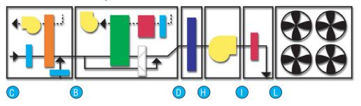
*ENTHALPY WHEEL*—The outside air is drawn through filters and the enthalpy wheel first. The leaving air condition of the enthalpy wheel is a product of the wheel efficiency and the enthalpy difference of the two airstreams. Select the enthalpy wheel efficiency from the Enthalpy Wheel Selection Chart in the Appendix.
